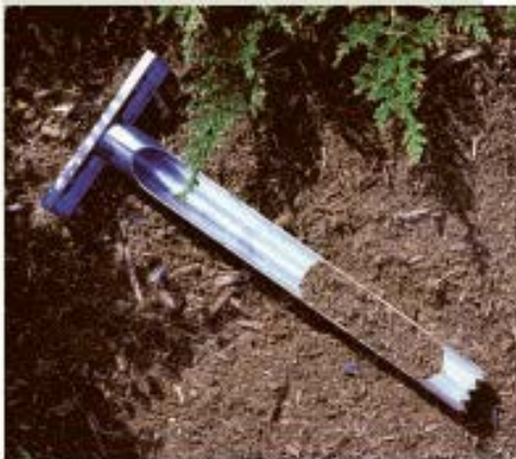
A LaMotte soil sampling tube with a saw-toothed cutting edge. This model takes a one-inch core sample to a depth of 10 inches.
