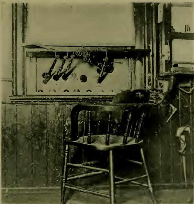
THE OBSERVATION ROOM, SHOWING TELESCOPES TRAINED ON FEEDING-STATIONS OR PERCHING-PLACES, AND PUSH-BUTTONS CONNECTED WITH ELECTRIC RELEASE ON CAMERAS
